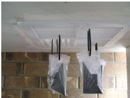
Side View showing flush to ceiling fit under pressure after 5 weeks of weight testing.
