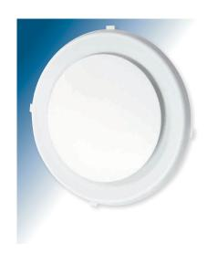
The standard Polyaire Round Ceiling Diffuser is manufactured from high impact ABS for long term strength and rigidity. It is fully adjustable by rotating the centre cone from total shutoff to fully open.
