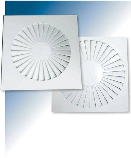
The Polyaire PSC Swirl Diffuser has fixed blades that create rotational as well as axial, tangential and radial air movement. This means that it produces a strong horizontal swirl, obtaining high inductivity, to allow the introduced flow to rapidly mix with the ambient air to reduce temperature and also perceived drafts or hot/cold spots.
