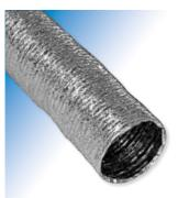
Polyaire Metallized Core fire rated flexible duct is manufactured from metallized Mylar and clear Mylar substrates, incorporating totally encapsulated helically wound spring wire. Bonded with a fire retardant and slip resistant dry deposit adhesive, this duct construction ensures a long life span in all ambient conditions.
