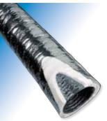
Polyaire Firebreak Flexible Duct is manufactured from metalized Mylar and clear Mylar substrates, incorporating totally enclosed helically wound galvanised high tensile steel wire. The layers are bonded with a fire retardant adhesive to ensure long life in all ambient conditions.
