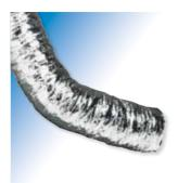
Polyaire Silentflex fire rated flexible duct is manufactured from metallized Mylar and clear Mylar substrates, incorporating totally encapsulated helically wound spring wire. Bonded with a fire retardant and slip resistant dry deposit adhesive, this duct construction ensures a long life span in all ambient conditions.
