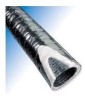
Polyaire Firebreak Flexible Duct is manufactured from metalized Mylar and clear Mylar substrates, incorporating totally enclosed helically wound galvanised high tensile steel wire. The layers are bonded with a fire retardant adhesive to ensure long life in all ambient conditions.
